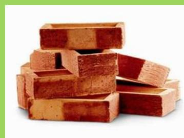
*Bricks made of sludge*
